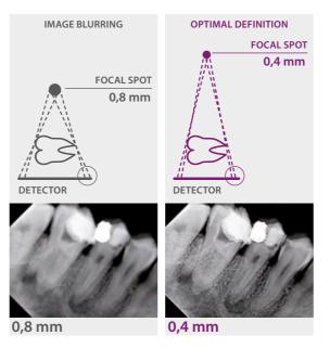
The constant potential high frequency generator (DC) provides sharp images with the very highest level of detail. Compared to AC systems, they also reduce exposure times and the amount of harmful radiation by containing the dose administered to the patient. A focal spot of just 0.4 mm - one of the smallest available - ensures images are always sharp and of the highest quality.
